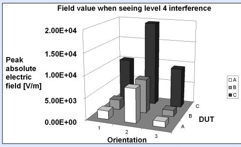
**Failure level 4** (Crash, Operator intervention) for GPS receivers for different orientations. Mono pulse. Peak electric field.
