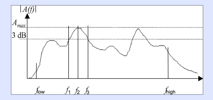
Note: 3 dB bandwidth does not represent the range of frequencies over which 90% of the waveform energy is found.
