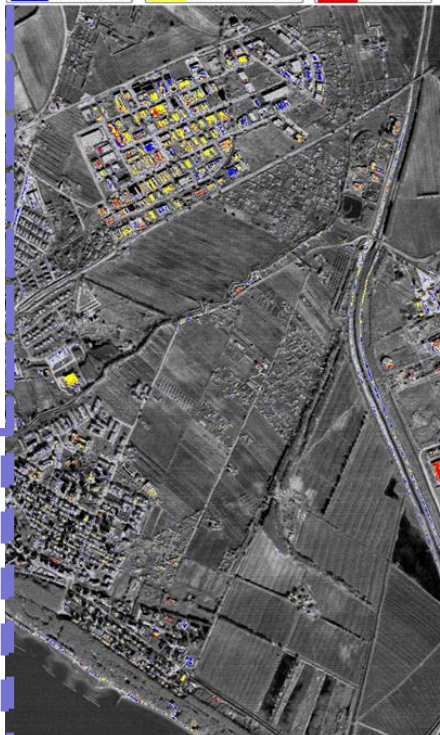
AC deterioration status map in the Follonica industrial area using MIVIS airborne data
