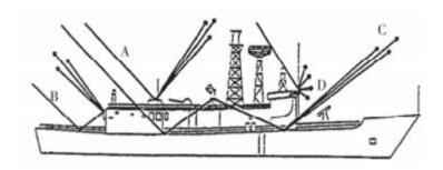
A = Single reflection C = Triple reflection B = Double reflection
